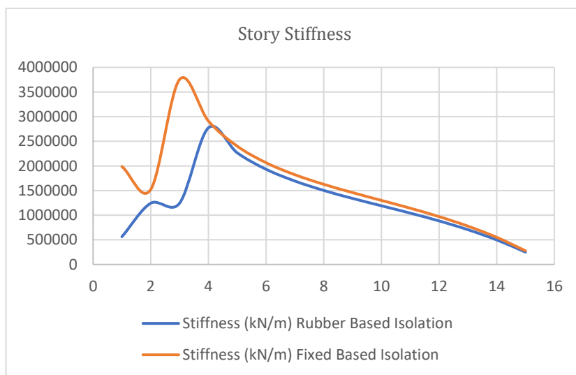
Figure 06. Showing values of Story Stiffness
