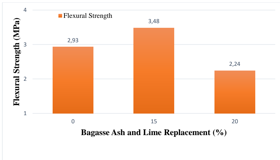
Figure 3: Graph showing flexural strength of concrete with respect to different % of Lime and Bagasse Ash
