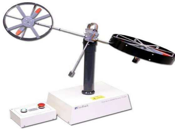
Figure 1. Twin rotor aerodynamic system [11].
