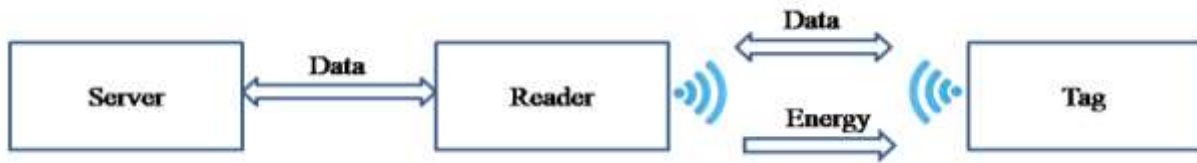
Figure 1. Basic RFID System
