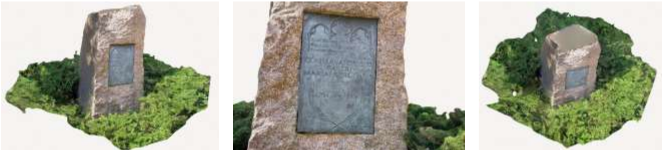
Fig. 2 Example of a partial 3D model created from 114 photos. On the right you can see that the top photos were missing. 3D model available: https://skfb.ly/oTC8C
