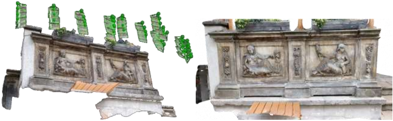
Fig. 1 3D models created using Pix4Dmapper Pro software in left and on the right using Polycam tools. On the left, the camera locations during object capture are shown.
