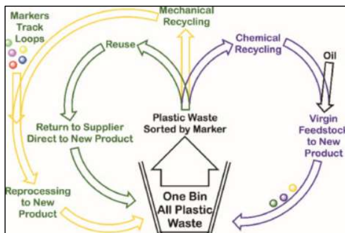
Fig. 1: Imagining the flow of plastics within the framework of the 'One Bin
