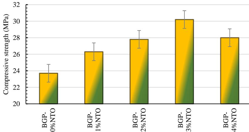
Fig 1. CS and compressive loads of FRF-GP mortar for different dosages of Titania
