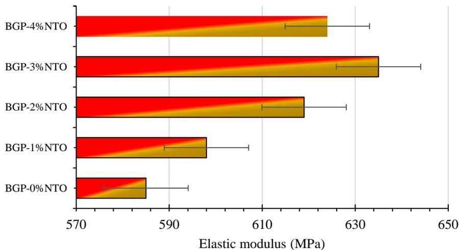
Fig 3. Elastic moduli of FRF-GP mortar for different dosages of Titania
