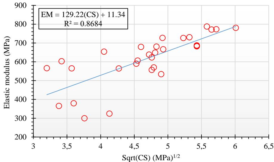
Fig 4. Relationship between CS and elastic modulus of GP mix
