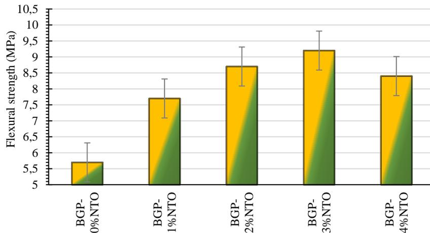
Fig 5. FS and bending loads of FRF-GP mortar for different dosages of Titania
