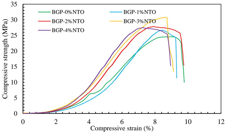
Fig 2. Compressive strength-strain behavior of FRF-GP mortar for different dosages of Titania
