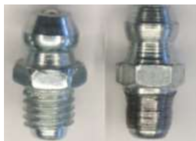
Fig. 7 OK/NOK grease fitting parts
