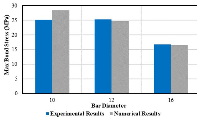
Figure 3: Numerical and Experimental Max Bond Stress Comparison for Rebars
