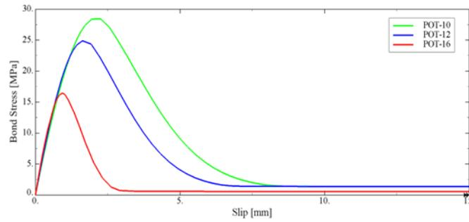
Figure 1: Comparison of Numerical Simulation Curves for 10mm, 12mm, and 16mm Rebars
