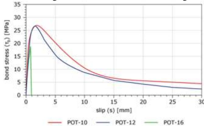
Figure 2: Comparison of Experimental Pull-Out Test Curves for 10mm, 12mm, and 16mm Rebars
