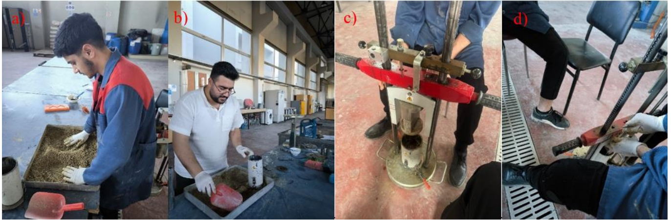
Fig. 3 MCV test stages a) Mixing b) compaction c) adjusting height d) measuring penetration
