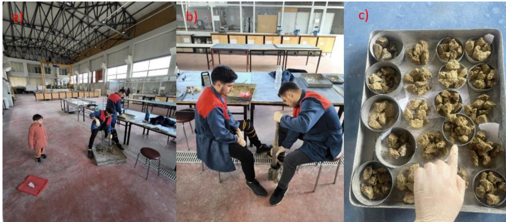
Fig. 2 Proctor test stages a) Mixing and compaction b) compaction c) moisture cans for water content
