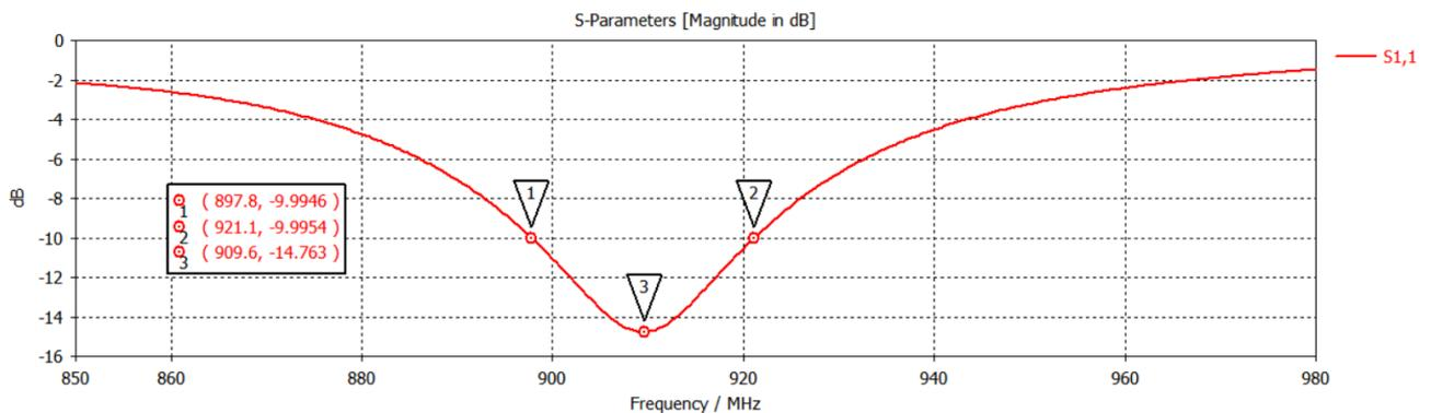
Figure 3: S Parameter of the Antenna
