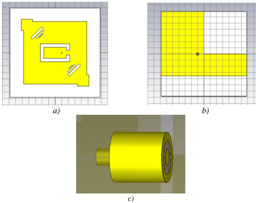
Figure 1: a) Front of the Antenna b) Back of the Antenna c) Feed of the Antenna
