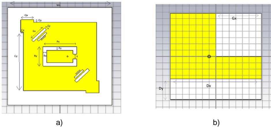
Figure 2: a) Front b) Back of the antenna with parameters
