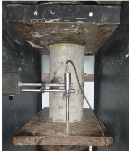
Figure 4. Testing of samples under axial compressive
