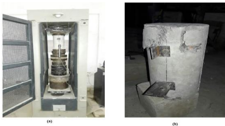
Fig. 4 : Compressive strength test on cylindrical specimens
