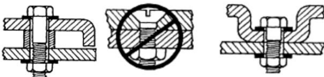
Figure 3. Bolts-Nuts connections in load-bearing applications
