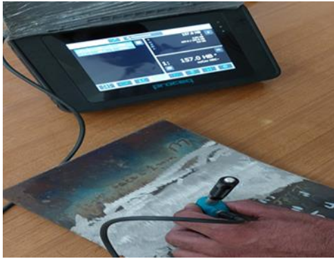
Fig. 6 Hardness Testing with Portable Hardness Tester
