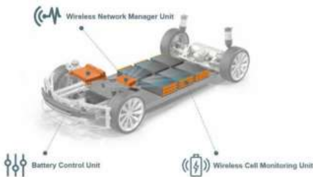
Fig. 1 The BMS system
