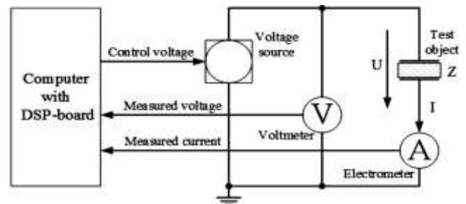
Fig. 2 FDS measurement circuit diagram of the oil paper insulation system of transformer
