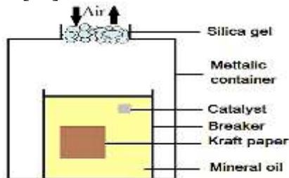
Fig. 3 Schematic representation of aging vessel.
