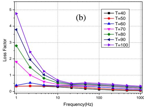
Fig. 7 Loss factor of aged kraft as function of the frequency for different temperatures (a) low frequency (b) high frequency
