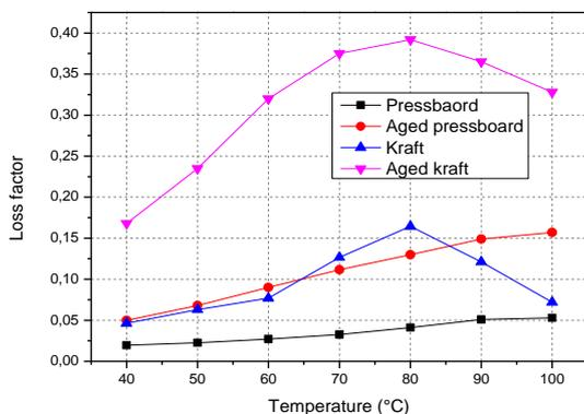
Fig. 8. Comparison of loss factor of papers at 50Hz as function of temperature
