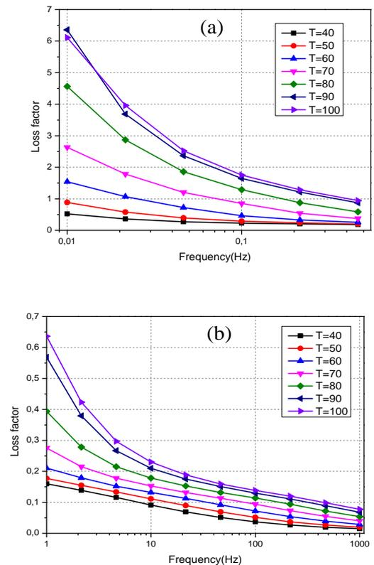
Fig. 6 Loss factor of aged pressboard as function of the frequency for different temperatures (a) low frequency (b) high frequency
