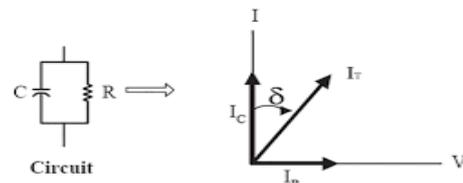
Fig. 1 Phasor diagram and equivalent circuit of a dielectric
