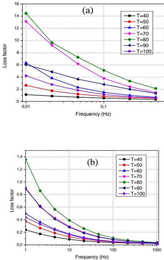
Fig. 5 Loss factor of kraft as function of the frequency for different temperatures (a) low frequency (b) high frequency
