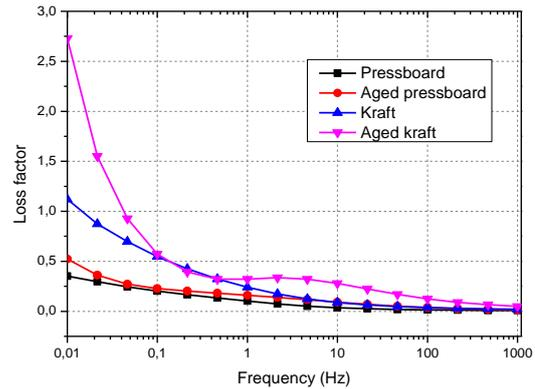
Fig. 9. Comparison of loss factor of papers at 40°C as function of different frequency
