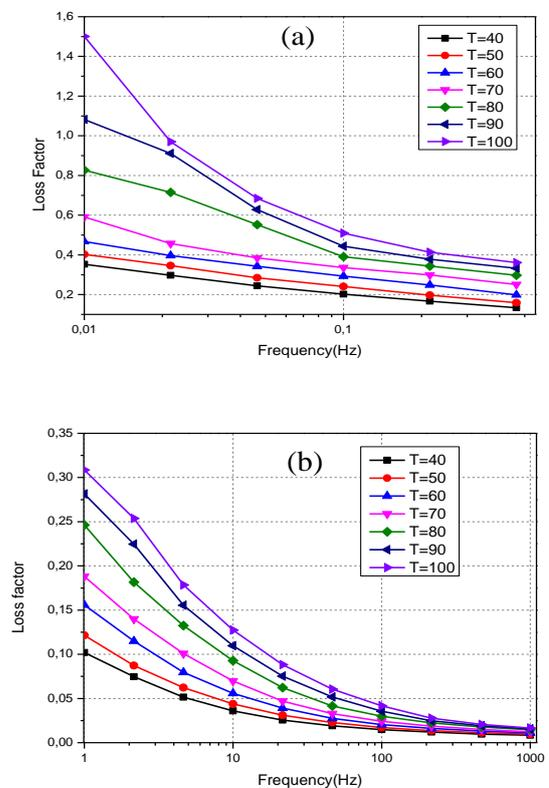
Fig. 4 Loss factor of pressboard as function of the frequency for different temperatures (a) low frequency (b) high frequency
