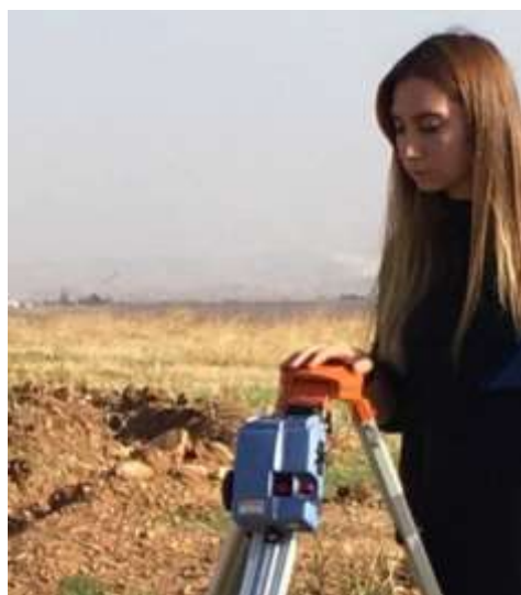
Figure 5. An image during measurement with Thermo Scientific Personal DataRAM pDR-1500 device
