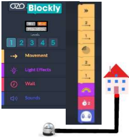
Fig. 4 The program code of the task solution in OzoBlockly programming environment and the task illustration [2]
