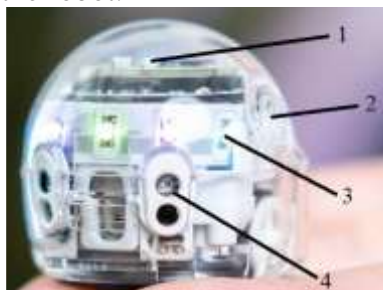
Fig. 1 1 – Status LED, 2 - on / off button, 3 - charging indicators LEDs, 4 – optical sensors.
