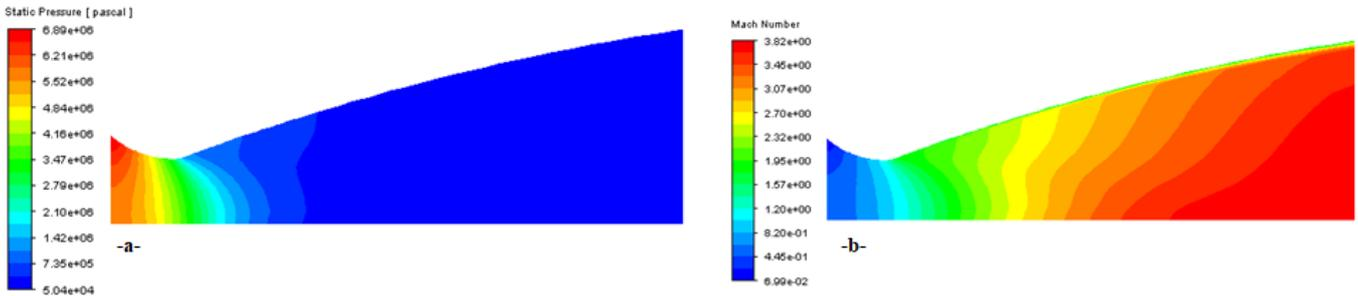
Fig. 6 contour plots of (a) static pressure and (b) Mach number along the nozzle
