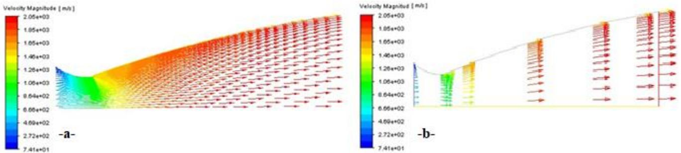
Fig. 7 Velocity distribution along (a) centerline and (b) cross-sections
