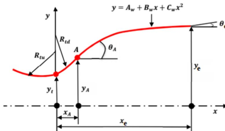
Fig. 1 Bell-shaped nozzle profile contour
