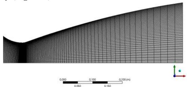
Fig. 4 Quadrilateral structured mesh
