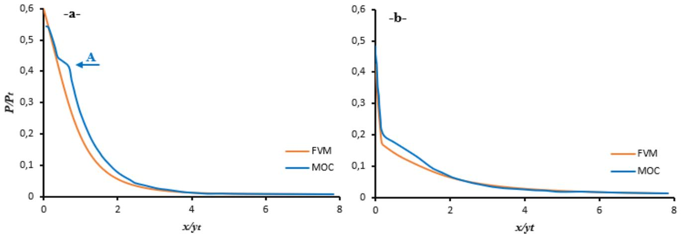
Fig. 5 MoC and CFD solutions in terms of static pressure along (a) centerline and (b) wall
