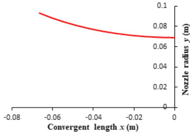
Fig. 3 Profile of the nozzle's convergent section
