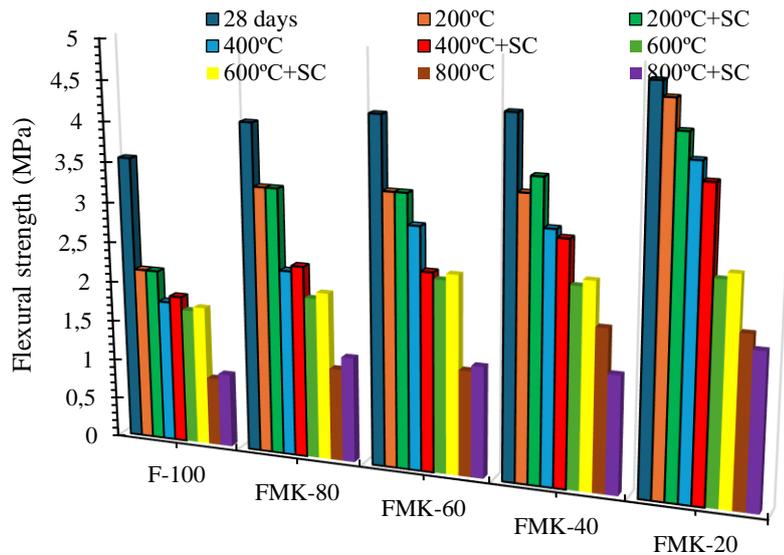
Figure 4. Flexural strength values of specimens for elevated temperatures subjected to SC and comparison with 28-days strength
