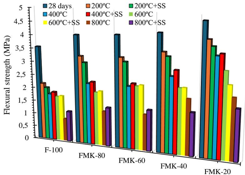
Figure 3. Flexural strength values of specimens for elevated temperatures subjected to SS and comparison with 28-days strength
