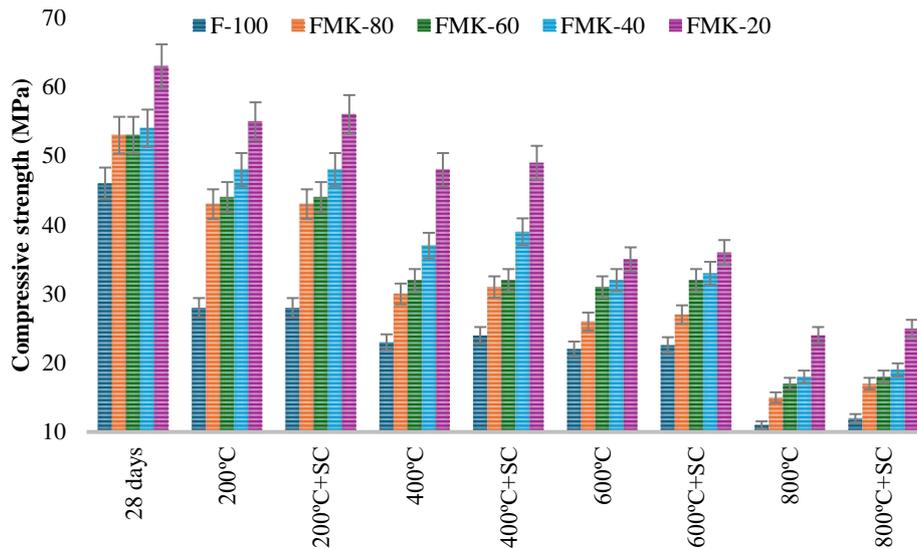
Figure 2. CS values of specimens for elevated temperatures subjected to SC and comparison with 28-days CS
