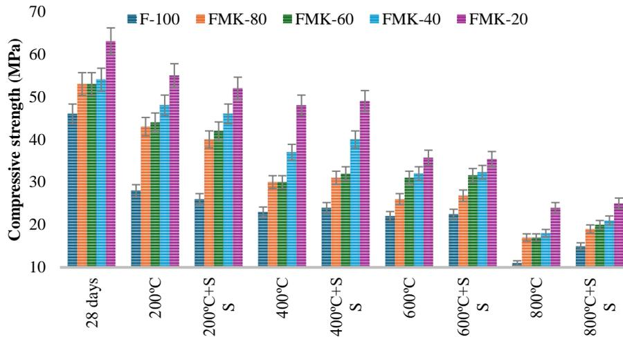
Figure 1. CS values of specimens for elevated temperatures subjected to SS and comparison with 28-days CS
