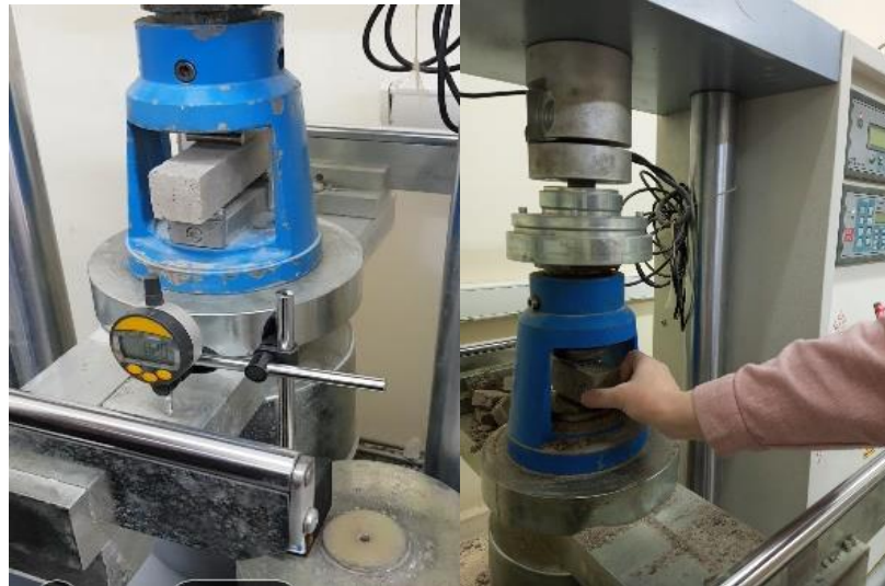
Figure 2. Flexural tensile strength (left) and compressive strength (right) tests
