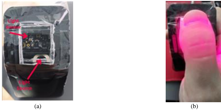
Figure 2: Proposed hardware setup - (a) General view of the system and (b) Finger placement for data collection
