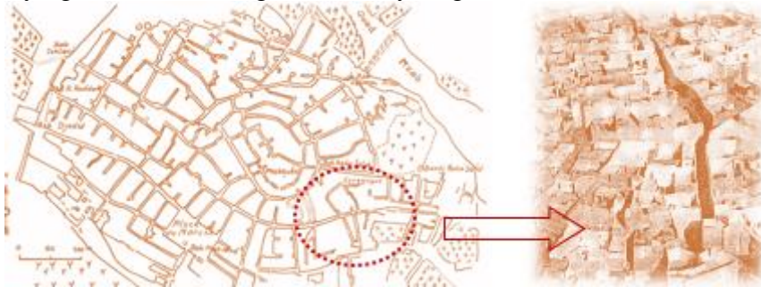
Fig.11: Shading effect created by east-west oriented streets in the village of Melika, Mزاب Valley. Source: Bennadji Amar, 1999.
