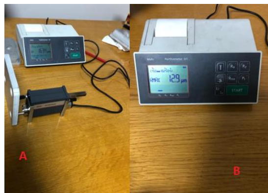
Figure 7 A: Test specimen Ra measurement, B: Surface roughness measurement device
