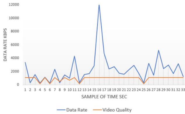
Fig 4: Data rate fluctuations and corresponding AI-based resolution adjustments during network testing.
