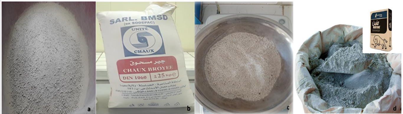
Fig. 1 Materials: a/ silty soil, b/ lime, c/ plastic waste, d/ cement
