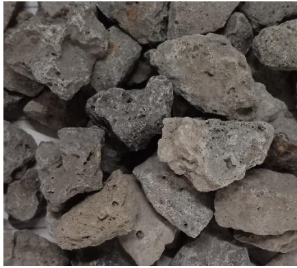
(a) Figure 1. Steel slag aggregates (a) image (b) granulometric analysis
