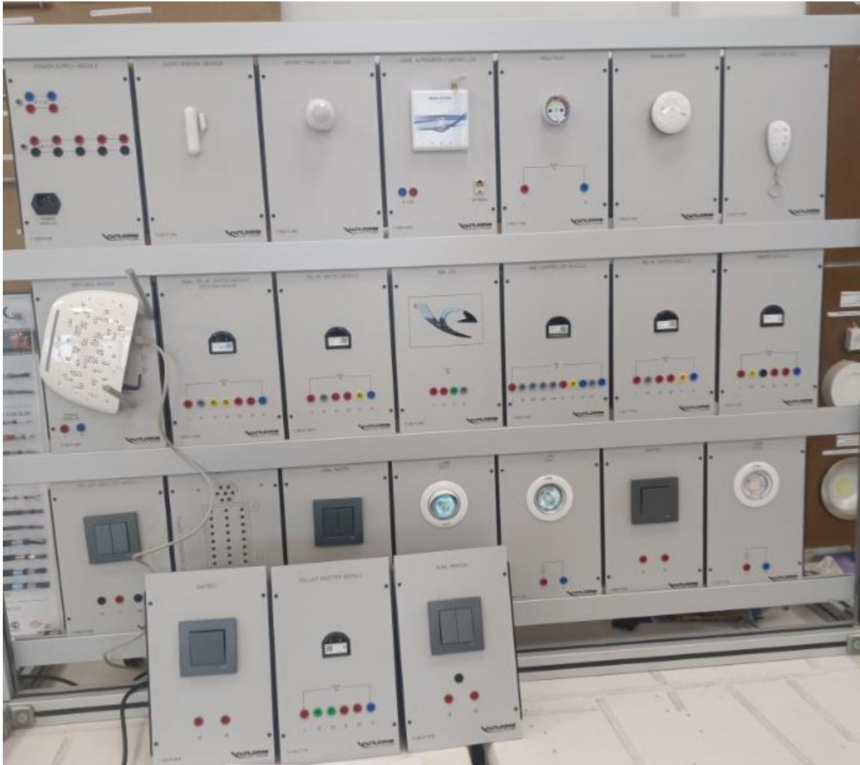
Fig. 5. Smart building automation systems application kit
