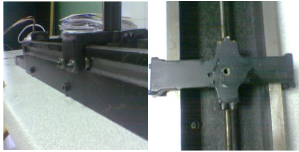
Fig. 3 Photos of the side carrier rail and main body carrier system mechanism of the new design opto-mechanical system.
