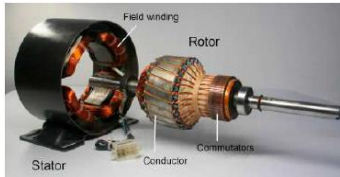
Fig. 2 Energy conversion in a DC motor.
