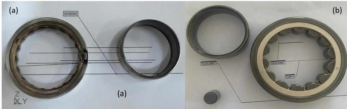
Fig. 2 Bearings a) motor bearing b) track bearing
