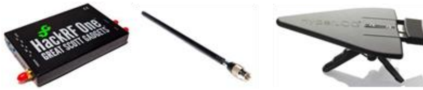
Fig. 2. Measurement materials: Left: HackRF One transceiver, Middle: Original HackRF dipole antenna Right: Log-periodic (HyperLOG) directional antenna.
