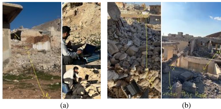
Fig. 3. (a) 1 st where Tx located at the center of the collapsed building, (b) 2 nd site where Tx located at a corner of the collapsed building.
