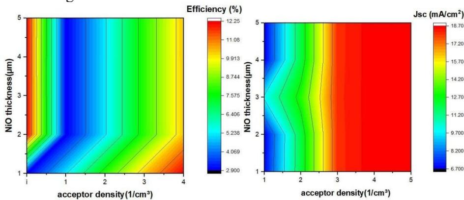
Figure 3  $J_{sc}$  and PCE of NiO thickness and acceptor density
