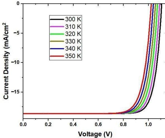
Figure 8 J-V curves with various temperature
