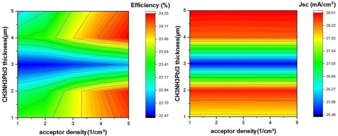
Figure 5  $J_{sc}$  and PCE of Perovskite layer thickness and acceptor density
