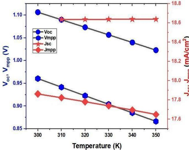
Figure 9  $V_{oc}$ - $V_{mpp}$  and  $J_{sc}$ - $J_{mpp}$  with temperature
