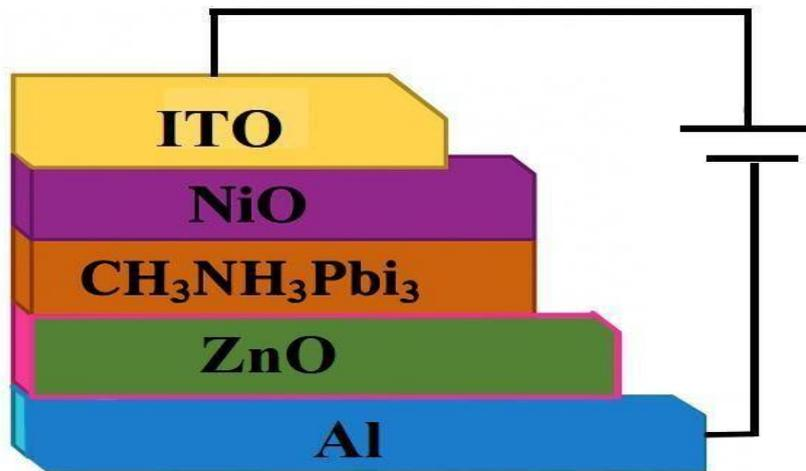
Figure 1 Schematic of the fabricated ZnO-based perovskite solar cell
