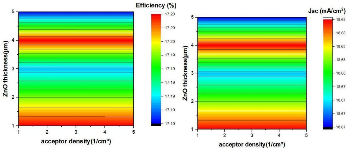
Figure 6 Jsc and PCE of ZnO layer thickness and acceptor density
