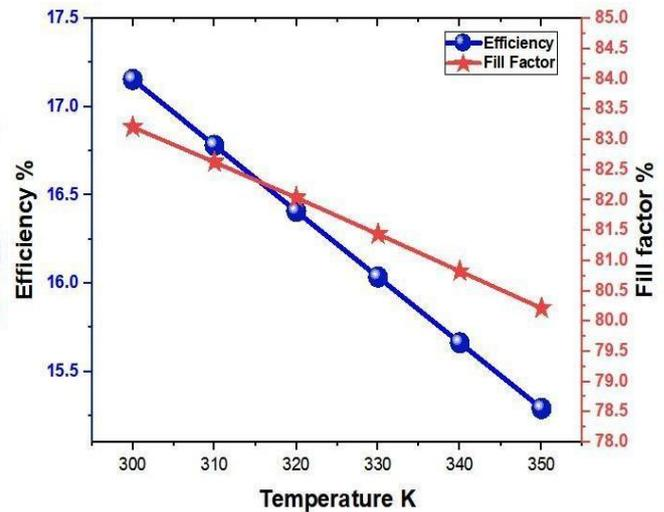
Figure 10 Efficiency and Fill factor with temperature
