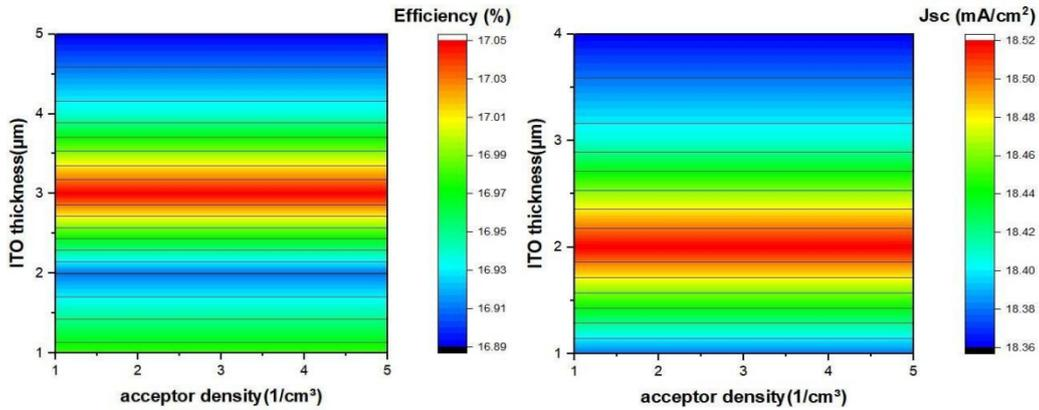
Figure 4  $J_{sc}$  and PCE of ITO thickness and acceptor density
