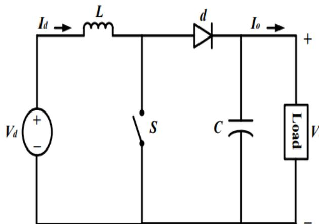
Figure 5: Equivalent circuit diagram of the DC-DC boost converter.
