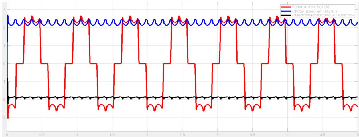
Figure 6. Stator Current, Rotor Speed, and Torque in PMSG
