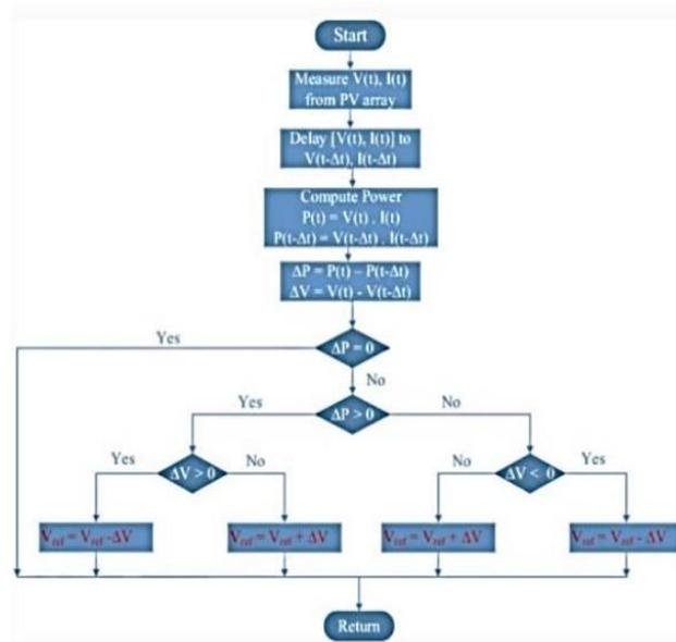
Figure 3: Flow diagram of P&O algorithm
