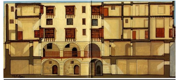
Fig. 7 section in Wikala Bazara showing different architectural elements in residential and commercial parts.
