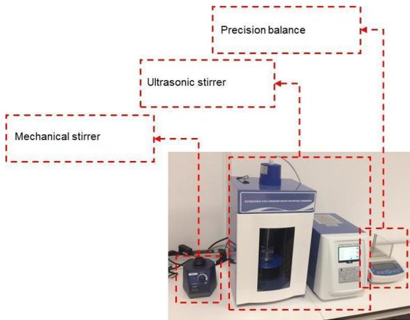
Fig. 2 Devices used in two-step method.
