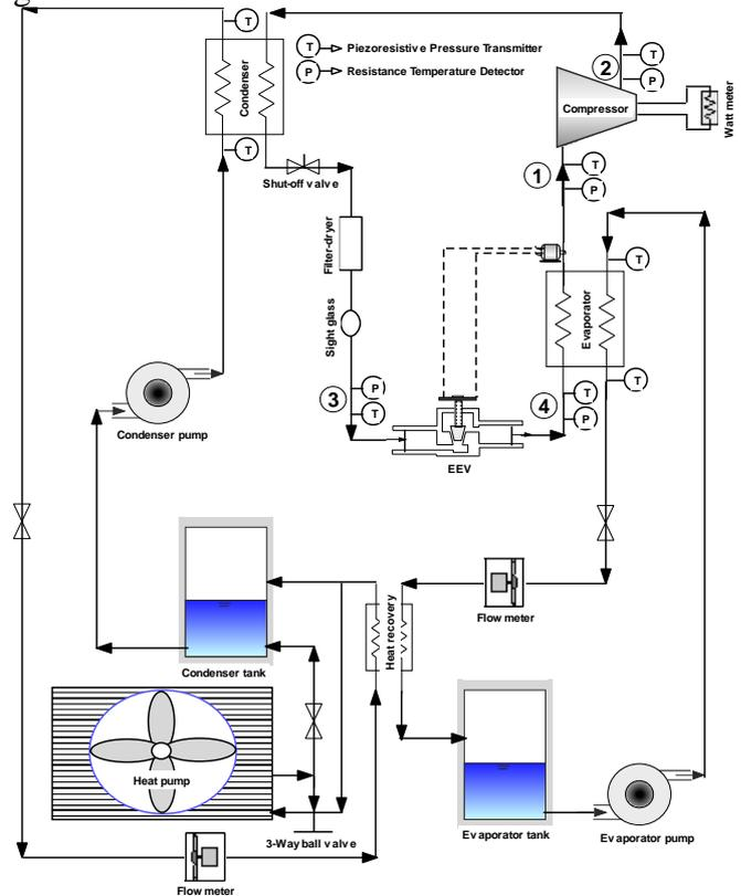
Fig. 1 Schematic representation of the VCRS test installation.
