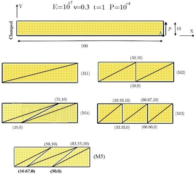
Figure 3. Beam in-plane bending (Data and meshes)
