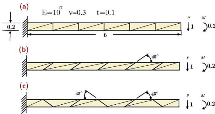
Figure 2. McNeal's cantilever beam (a) rectangular (b) trapezoidal (c) parallelogram
