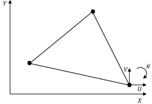
**Figure 1:** Strain Based Three node element
