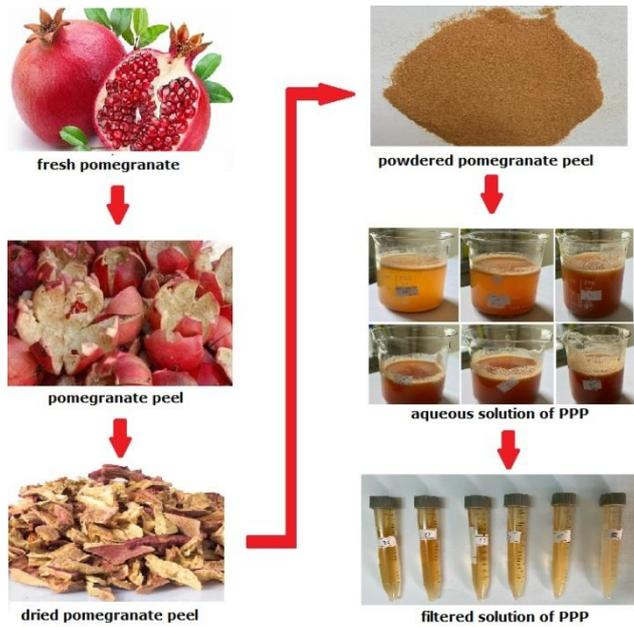
Figure 2. Preparation steps of PPP solutions before rheological measurements
