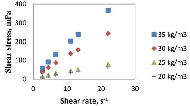
Figure 3. The plot of shear rate and shear stress for different concentrations of PPP
