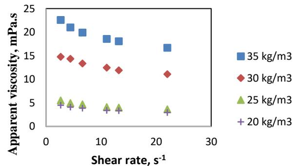
Figure 4. Variation of apparent viscosity with the shear rate for different PPP concentrations
