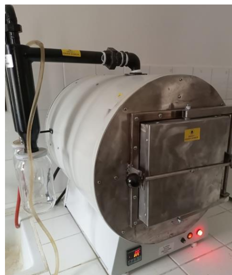
Figure 1. PID-controlled pyrolysis reactor system
